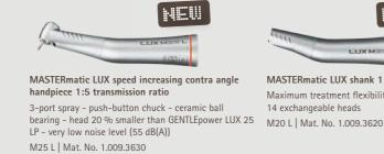
MASTERmatic LUX speed increasing contra-angle 1:5 transmission ratio Miniature head specifically for short-shank burs - 1-port spray - push-button chuck - ceramic ball bearing - head 43 % smaller than GENTLEpower 25 LP - very low noise level (55 dB(A))
