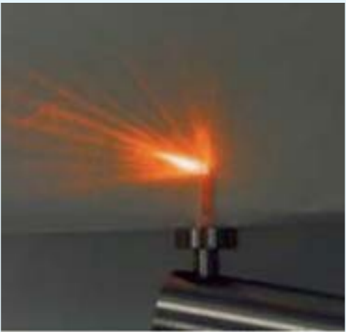
100% deflection of the laser beam by the prism.
