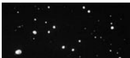
Note the number and size of voids in this thin film of cement mixed in a conventional shaker-type capsule mixing unit for 10 seconds.
