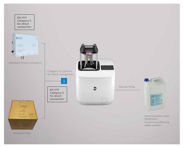
Direct connection: A water filter (20 μm) must be installed upstream of DAC Universal / DAC Universal S to ensure that the water is clean. This serves to protect your DAC Universal / DAC Universal S. REF. 63 12 214
