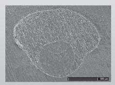
The SEM cross-section of a canal filled with GuttaCore shows a complete fill. All gutta-percha
