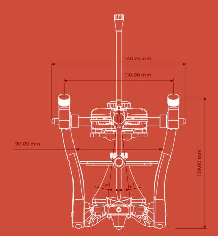
5050 and 5050Plus are non-Arcon average value articulators designed to help dental technicians meet dentists' requests for high precision regardless of the prosthetic technique. A light, stable and ergonomic construction facilitates set-up and work on any models. Additional features guarantee an exact simulation of the condylar path with a high fitting accuracy, giving prosthesis and restorations the necessary occlusion and function throughout the full range of mandibular movements.
