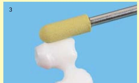
3 The round shape facilitates finishing of chamfers for individual abutments. This way the time for finishing is reduced and the efficiency is increased.
