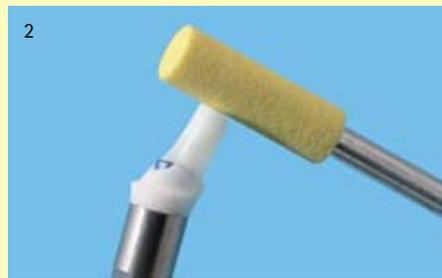
2 Processing without pressure and simultaneous cooling due to the diagen binding material avoid damage to the zirconium.
