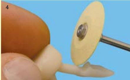
4 The unique diamond binding material ensures longer tool life and the coarser diamond grain facilitates efficient processing.
